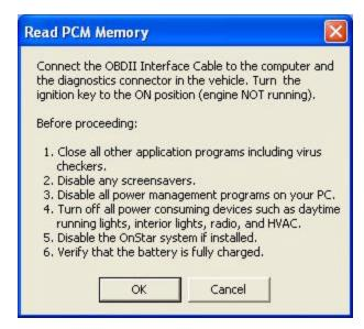
Before proceeding, connect the DST OBDII interface to your PC. Connect the other end of the converter to the ALDL diagnostics connector on the vehicle. (The ALDL connector is located under the dash on the driver's side.)
