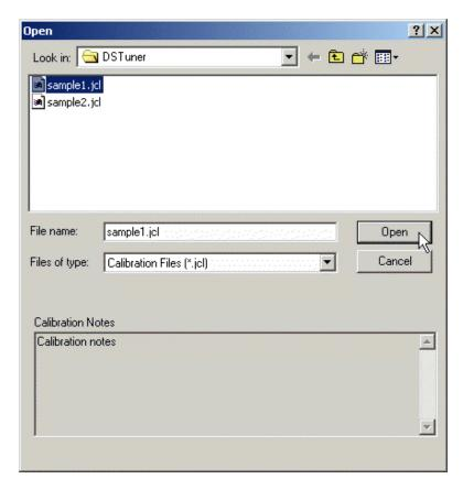
Select a calibration file and click on the '*Open*' button to load the calibration file into the DST program. When you click on a calibration file name in the Open File screen, any notes that have been saved with the calibration file will be displayed in the Calibration Notes box at the bottom of the screen.
