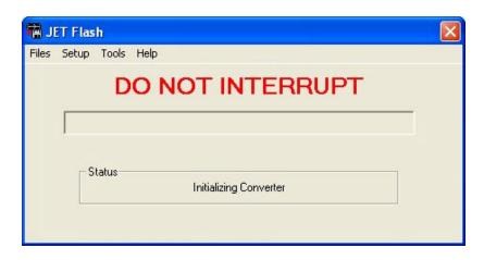
The progress meter shows the progress on the programming as it proceeds and the Status window describes what part of the process in currently underway. Depending on the PC you are using, the programming will usually take a minute or two.
