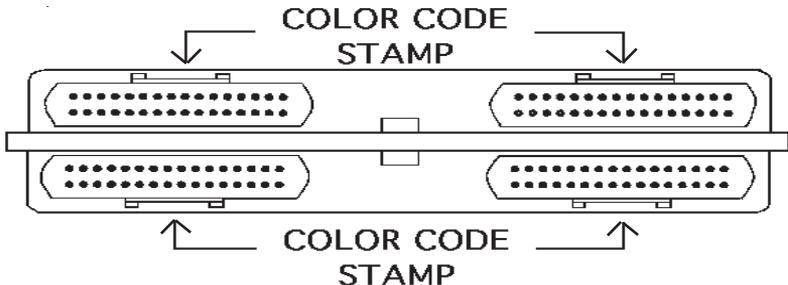
4. Notice on the ECM/Computer that each of the wire harness connectors is labeled with a separate color (ie: black, red, blue, white, etc.) This label may be stamped onto the metal housing of the ECM/Computer above where each wire harness connector plugs into the ECM/Computer.
