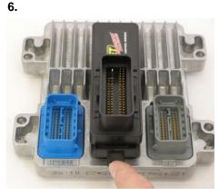
Step 5: Reinstall the computer on the firewall and reattach the connectors to the computer. Be sure to lock the connectors in place with the gray connector handles and the red securing straps. Reconnect the battery cable, then start the vehicle and make sure the check engine light is not on and the vehicle is running normally. This completes installation. Please keep these instructions for future reference.
