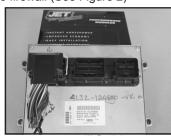
3. On your vehicles' computer you will find 3 wiring harnesses. Looking at the computer with all three plugs facing you, unplug the harness on the left by pulling back on the gray release bar. The module will back out of the computer and can be easily removed (See Figure 3).
