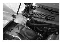
7. Disconnect the wiring connectors by pressing/squeezing down on the red release buttons on the top of the connector. Remove all the connectors from the ECU. (see photo 5)
