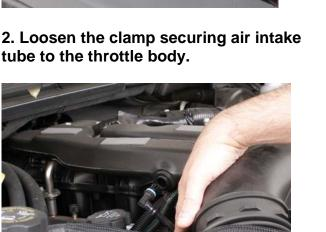
4. Disconnect breather tube from intake by gently pulling outwards. Loosen clamp at mass air sensor then remove intake tube.
