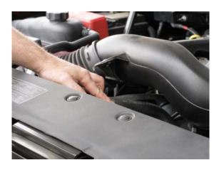
3. Disconnect air intake tube from radiator hose by gently prying on plastic clamp.
