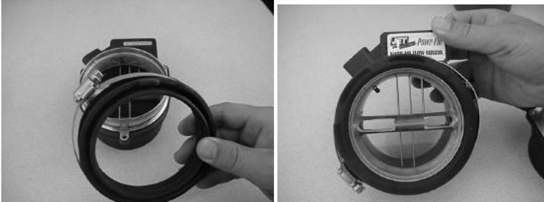
**4. Install JET Powr-Flo Sensor, tighten all clamps and plug in harness**
