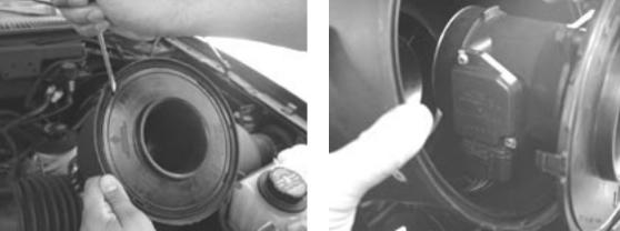
3. Remove stock Mass Air Sensor and Install Powr-Flo Sensor
