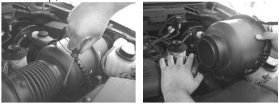
2. Open Mass Air Sensor Housing and disconnect Mass Air Sensor wiring harness
