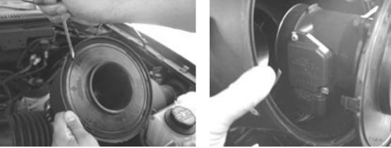
3. Remove stock Mass Air Sensor and Install Powr-Flo Sensor
