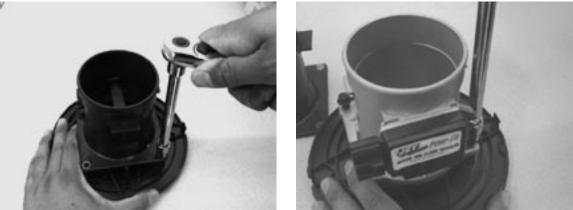
4. Reinstall into Mass Air Sensor Housing, reconnect wiring harness, close housing, reinstall onto intake, tighten all clamps
