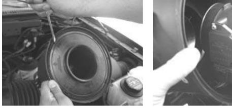
3. Remove stock Mass Air Sensor and Install Powr-Flo Sensor
