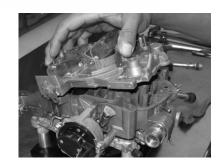
2. Using a hammer and punch, drive out the plug in the carburetor lid.
