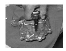
4. Use the supplied adjusting tool to set the APT(Adjustable Part Throttle) setting. This is best done with the carburetor installed, the engine running with the car fully warmed up. The APT can be used to help with throttle tip in issues by adjusting the screw up or down. Up is richer, down is leaner. The APT will have no effect on the idle, it is only used in the primary circuit, after the throttle blades begin to open.
