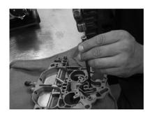
3. Using the supplied tap, thread the hole for the new pipe plug. Check the depth of the threads by installing the supplied pipe plug and making sure the new plug is level with the top of the carburetor. (It's ok if it goes below that, you just don't want to leave it sticking up or it will interfere with the air cleaner seating).
