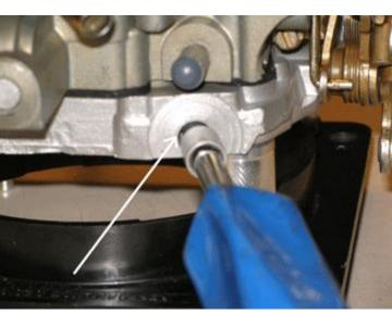
The imbedded idle fuel mixture screw is adjusted using either a 3/16 hex socket or a GM Double D adjustment tool. Turn the screw clockwise for a leaner mixture, counter clockwise for a richer mixture.
