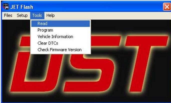
The program will then ask for a file name to give to the calibration file that will be created when the PCM is read.
