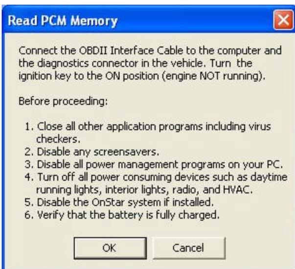
Before proceeding, connect the DST OBDII interface to your PC. Connect the other end of the converter to the ALDL diagnostics connector on the vehicle. (The ALDL connector is located under the dash on the
