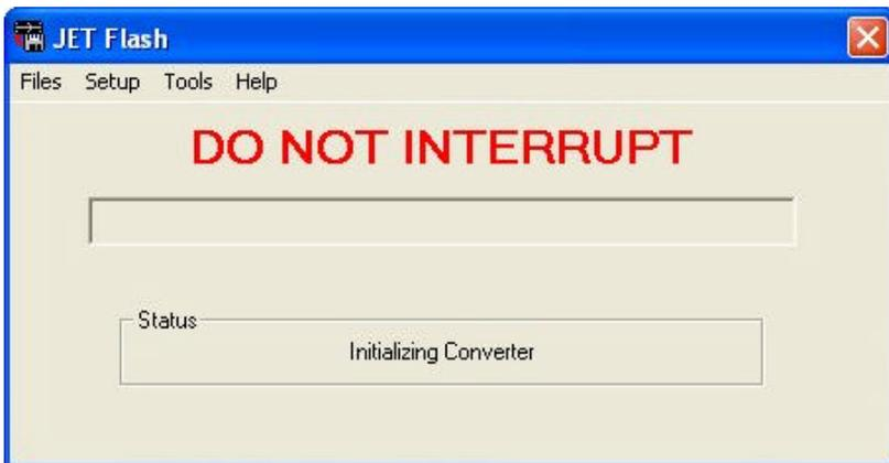
The progress meter shows the progress on the reading of the PCM as it proceeds and the Status window describes what part of the process is currently underway. Depending on the type of vehicle and the PC you are using, the read will usually take about four minutes.
