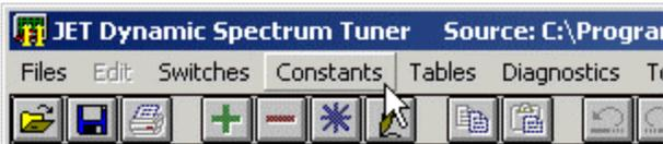
For example, to view constant type parameters, click on the 'Constants' menu. The constant parameters are then arranged in sub-groups according to function. When you click on one of the calibration parameter menus the sub groups are then displayed.
