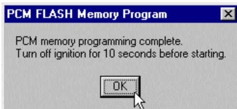
Click 'OK' to complete the PCM programming and close the Programming Complete message box. Your PCM is now programmed with the new calibration and ready for testing.
