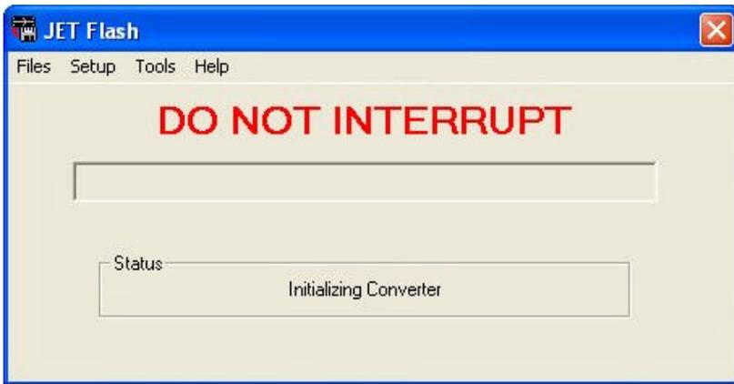
The progress meter shows the progress on the programming as it proceeds and the Status window describes what part of the process is currently underway. Depending on the PC you are using, the programming will usually take a minute or two.
