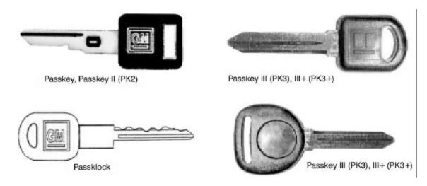
**Vehicle Anti-Theft System (VATS) & Passkey –** VATS and Passkey have a separate module called the Theft Deterrent Module (TDM) that validates the resistive chip in the ignition key. If the resistance value read by the TDM is what the TDM is expecting the TDM will send a signal to the PCM informing the PCM that a valid key is present and the PCM may start the vehicle. No relearn is required on a VATS equipped vehicle when replacing the PCM.
